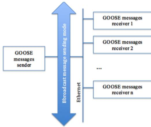
Figure 3 – Generalized scheme of GOOSE-messages transfer in an industrial computer network
