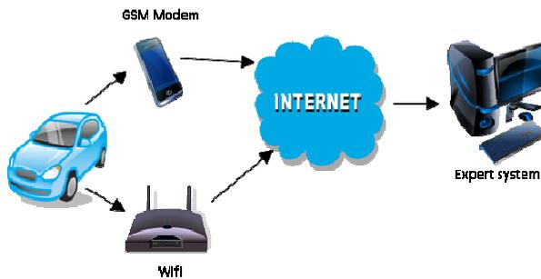
Figure 2 – Design of architecture for distant measurements in automobile
