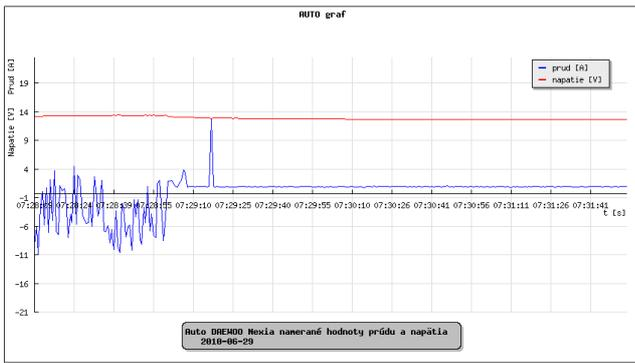
Figure 8 – Graphical representation of turning off the automobile
