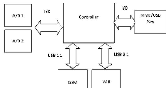
Figure 3 – A flow chart of the measuring chain
