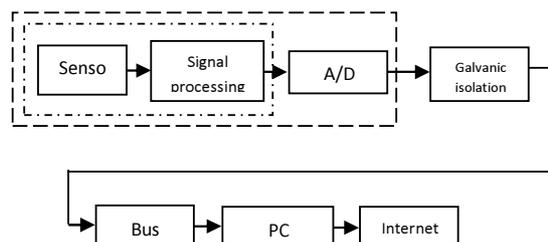
Figure 1 – Automated measurement chain
