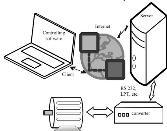
Figure 2 – Remote system architecture
