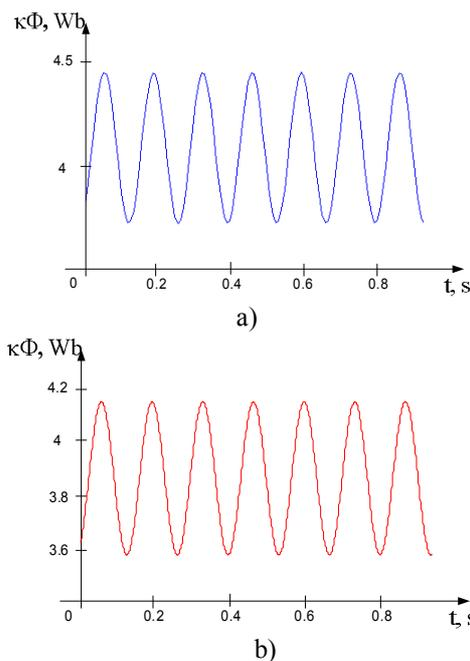
Figure 7 – Curves for  $k\Phi(t)$ : a) obtained by simulation; b) obtained by calculating
