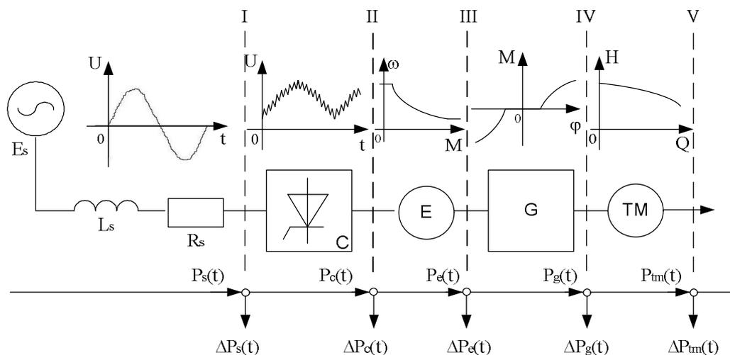
Figure 1 – The scheme of the energy conversion in electromechanical complex:
