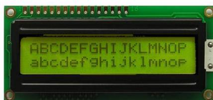
Figure 7 – 5 LCD Module 1602A-1
