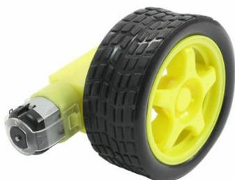
Figure 6 – DC motor with wheel
